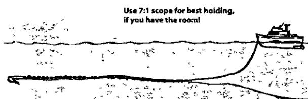
One myth we'd like to dispel is that a boat length of chain will keep the pull on an anchor shank parallel to the bottom. This is unfortunately not the case, since even a 15 knot wind will lift short lengths of chain clear off the bottom. Yes, it is better to use chain but, no, it isn't effective as windspeeds increase. Its primary mission is to handle the chafe from rough bottoms that would otherwise abrade the soft nylon line.
